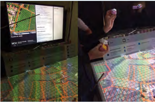
fig. 56 Movable blocks placed on the “Finding Places” urban visualization tool (left); characteristics of a plot projected onto the screen and shown to participants in a “Finding Places” workshop (right).
