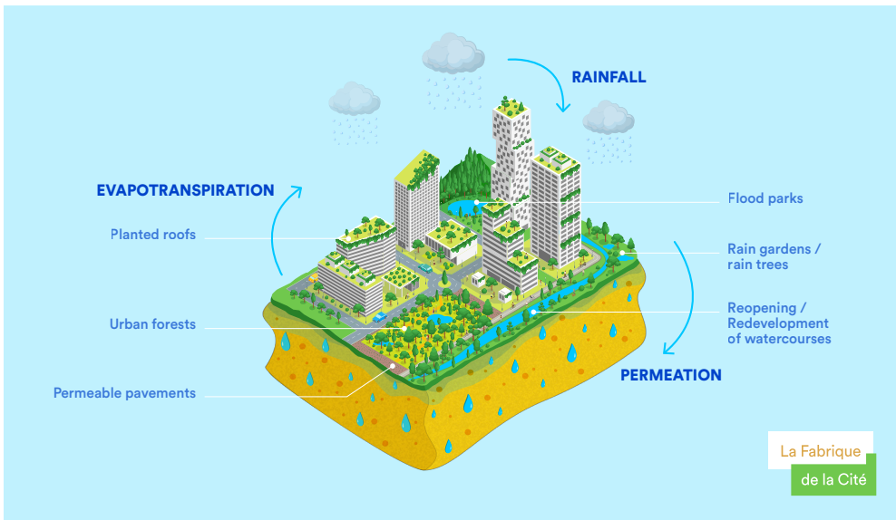
Conceptual diagram of a sponge city showing the processes enabling water absorption and reuse.
